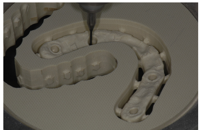
Fig. 3. Fiber-composit disk during milling process. After the digital design, the project is realized through a milling machine.
